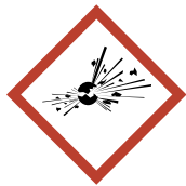
Explosion hazard (for explosion or reactivity hazards)
